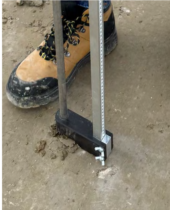
Figure 14: Inserting the DCP device in the layer.
