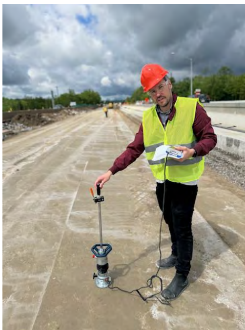
Figure 8: LWD device on Testing Site 1
