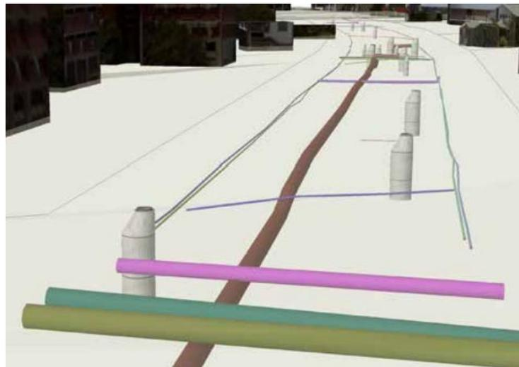
*Figure 12: 3D model of underground utilities in Zürich and Toa Payoh [12,13]*
