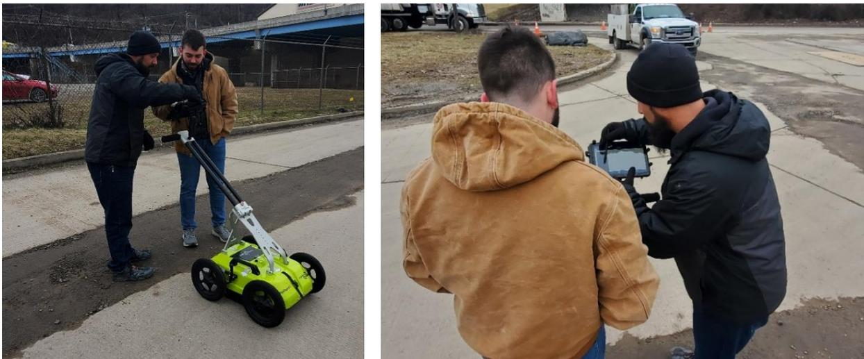
*Figure 55: PinPointR device used on the urban site*
