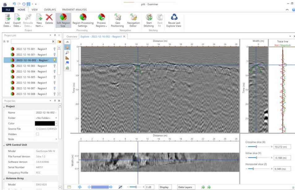
Figure 46: The above, A, and B scan shown in Examiner 3
