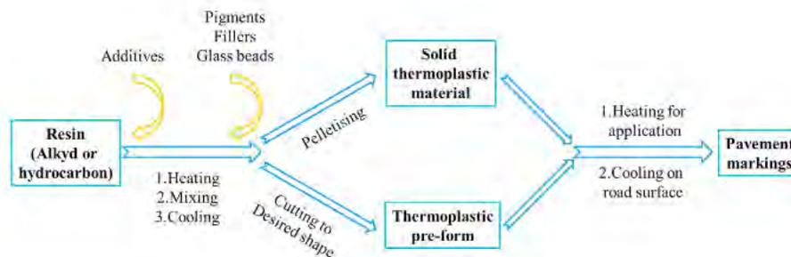
Figure 2: Thermoplastic processing for pavement marking application [1]
