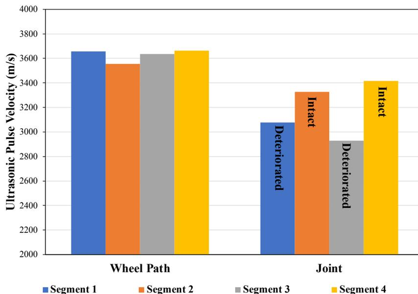
Figure 28: Ultrasonic pulse velocity at wheel path and longitudinal joint in Section 1
