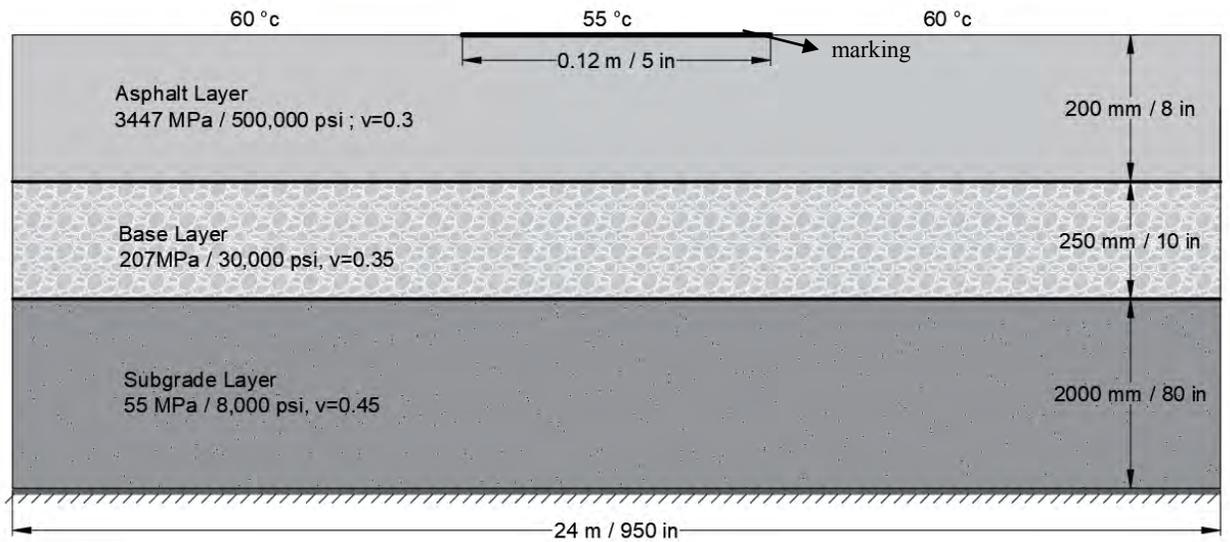
Figure 34: Three-layered asphalt pavement model
