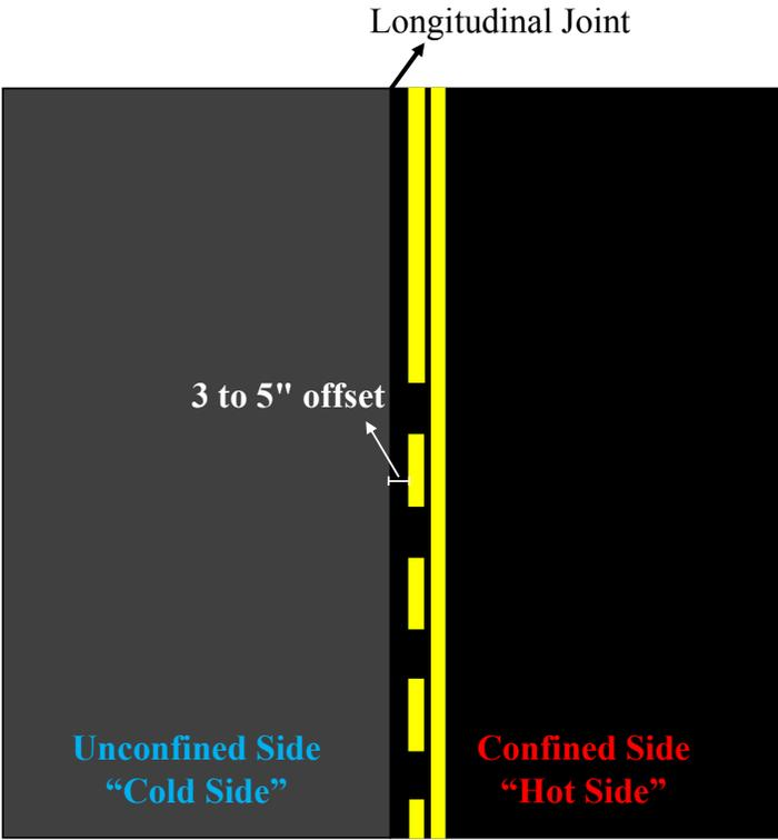
Figure 41: Suggested pavement marking placement
