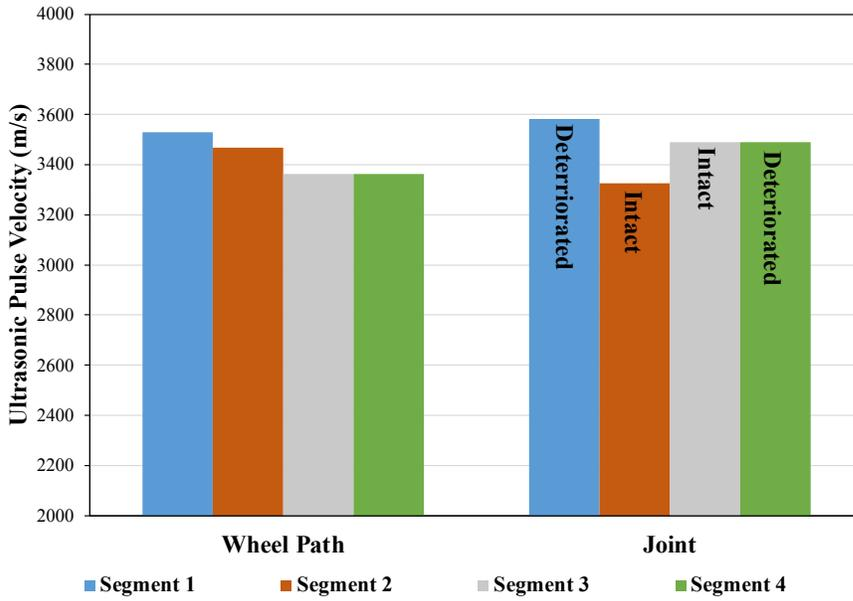
Figure 30: Ultrasonic pulse velocity at wheel path and longitudinal joint in Section 3
