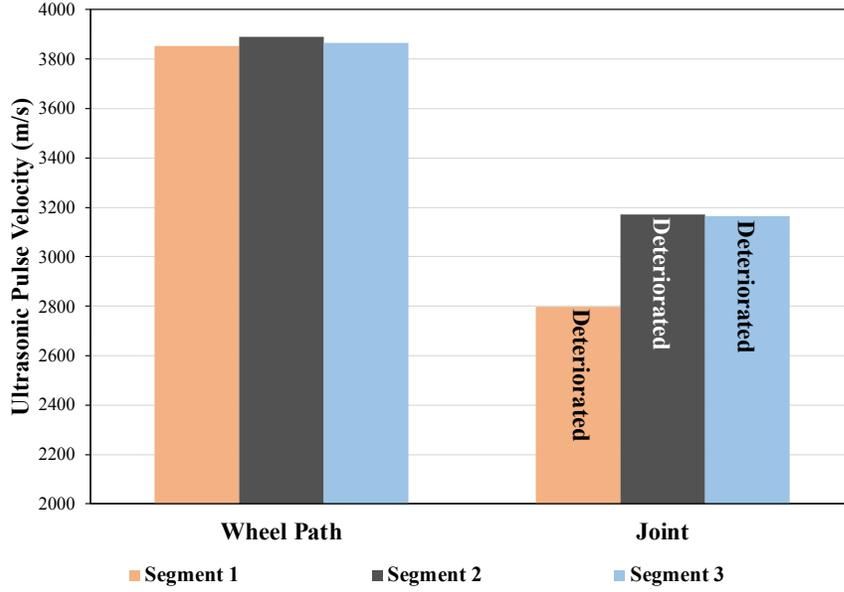
Figure 29: Ultrasonic pulse velocity at wheel path and longitudinal joint in Section 2
