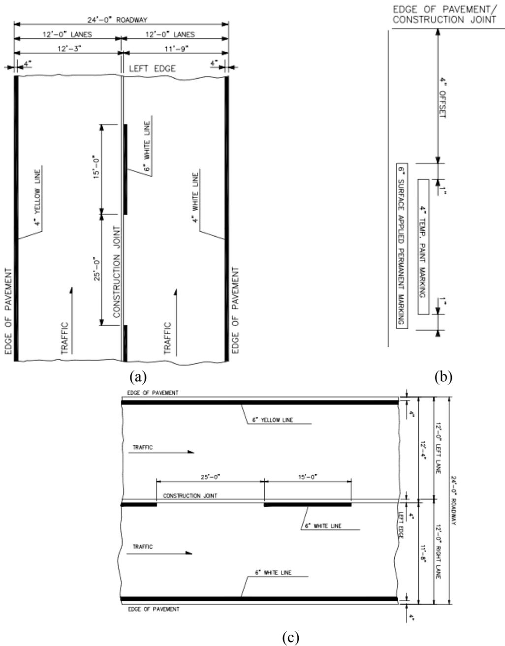
Figure 24: Turnpike Commission standards regarding offset of centerline marking placement from longitudinal joint in (a) 2011 [54], (b) 2012 [55], and (c) 2015 [56]
