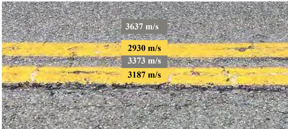
Figure 33: Ultrasonic pulse velocity at the longitudinal joint in different locations
