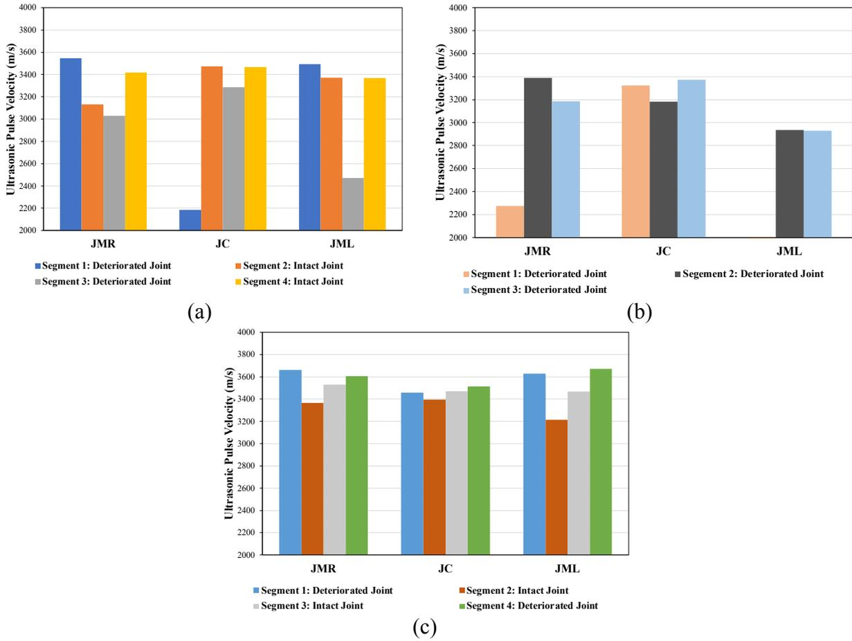
Figure 32: Ultrasonic pulse velocity at the joint for (a) Section 1, (b) Section 2, and (c) Section 3
