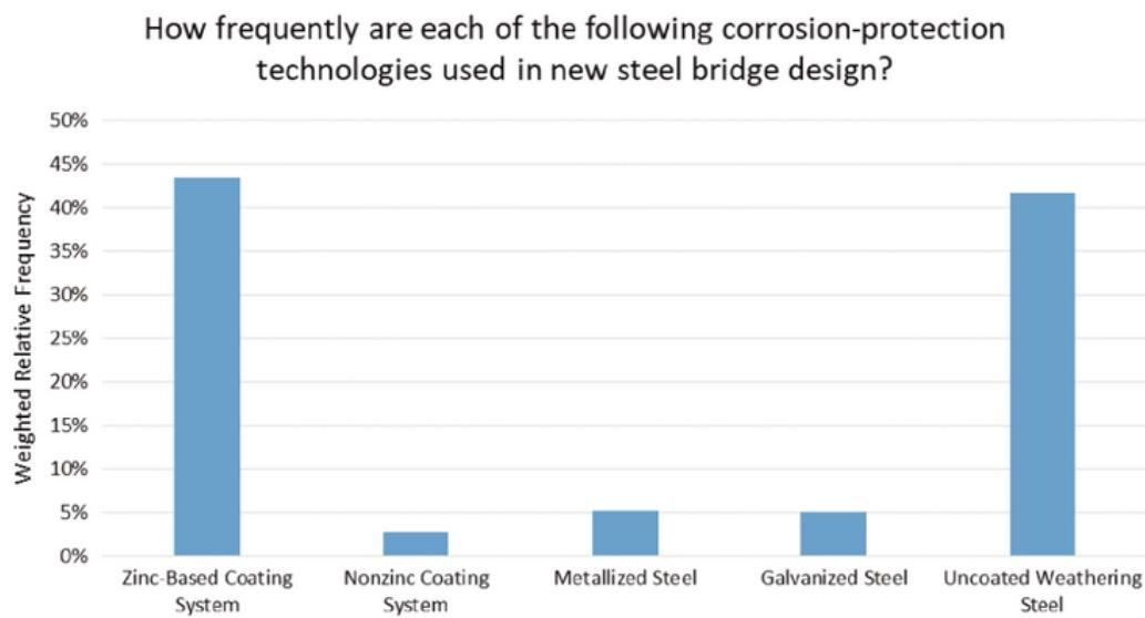
Figure 27 Corrosion protection technologies used for new steel bridges [44]
