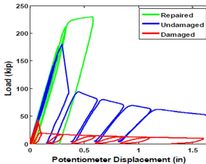
Figure 38 Force-displacement response of corroded girder repaired using UHPC encasement [58]
