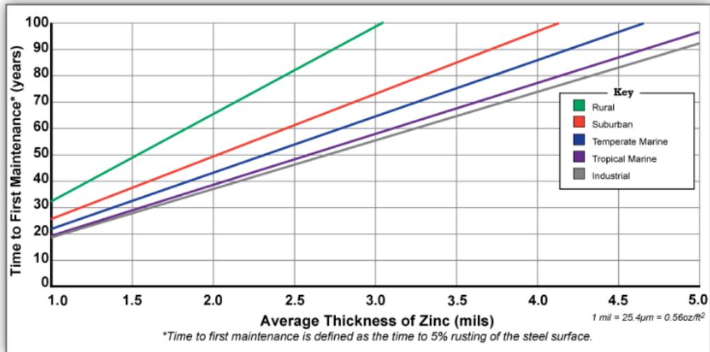
Figure 17 Lifetime prediction of galvanizing steels [19]
