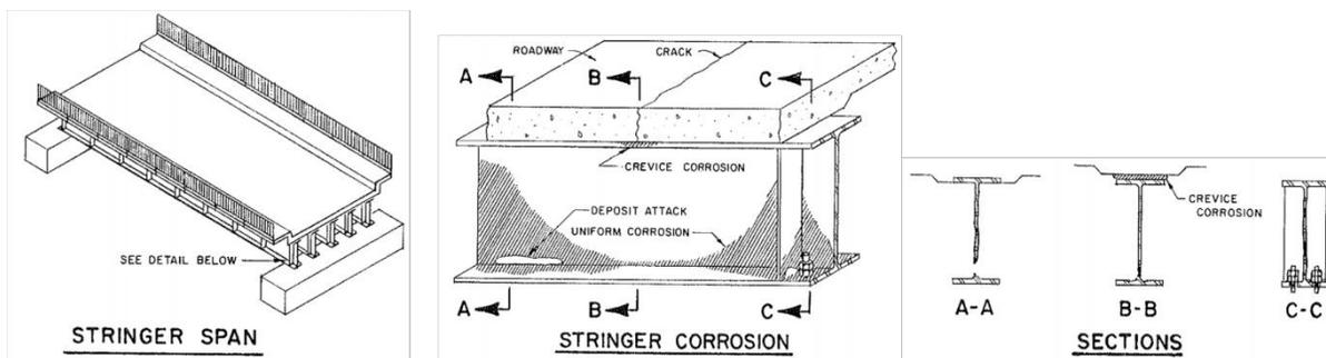
Figure 12. Common Corrosion Modes in Stringer Span Bridges [6]
