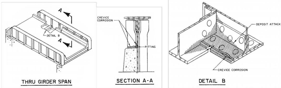
Figure 13. Common Corrosion in Through Girder Span Bridges [6]
