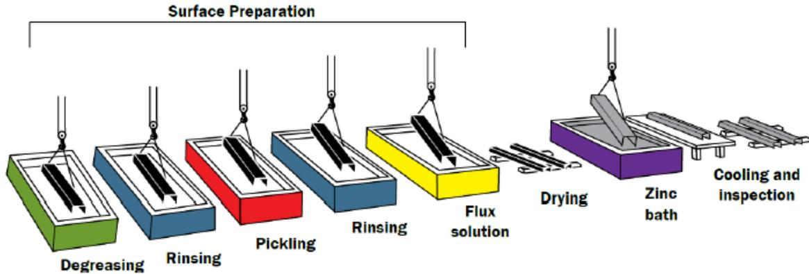
Figure 16. The hot-dip galvanizing process [17]
