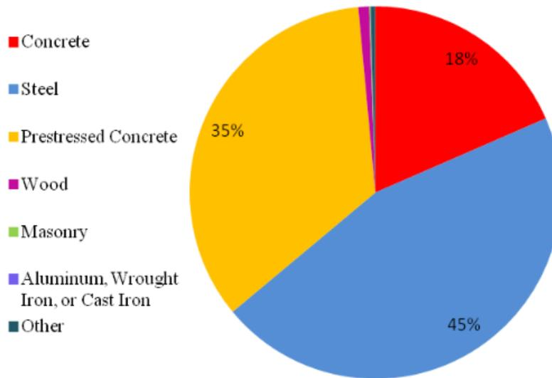
Figure 2. Distribution of Materials Used for Main Spans of US Highway Bridges, by Deck Area [3]
