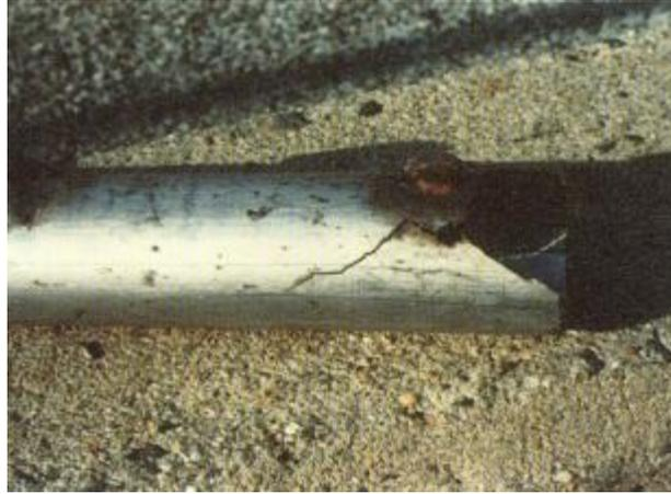
Figure 10. Stress Corrosion Cracking in Steel Pipe [6]
