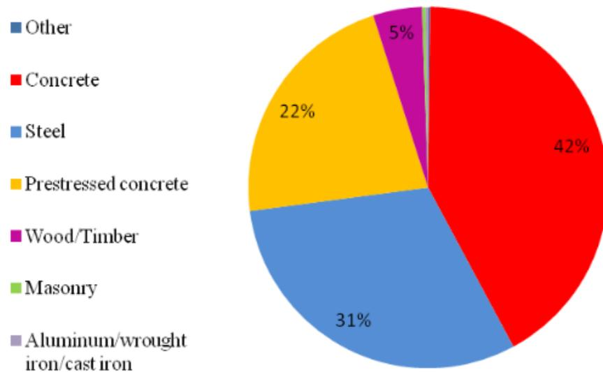
Figure 1 Distribution of Materials Used for Main Spans of US Highway Bridges by Number [3]
