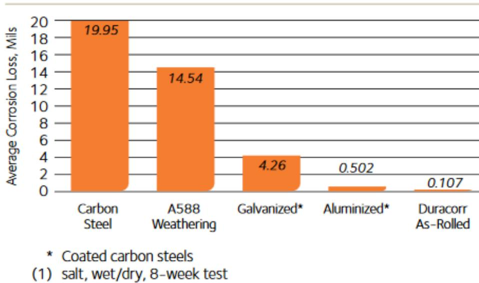
Figure 31 Corrosion Performance in SAEJ2334 Test [50]
