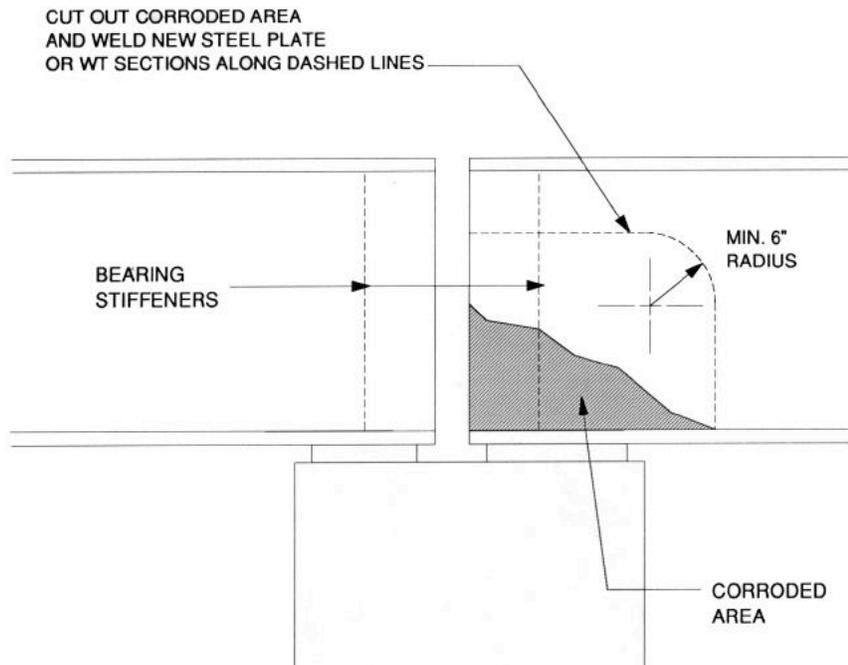
Figure 25 Corroded Steel Girder End Repair Detail [36]
