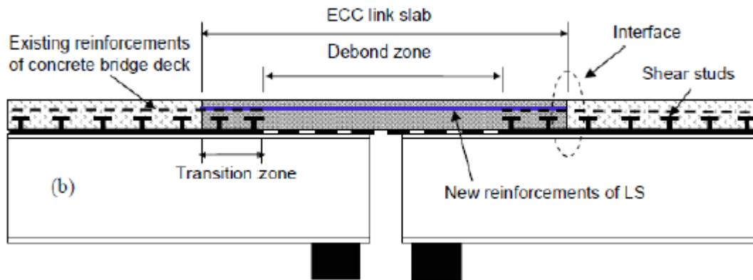
Figure 33 Debonded Link Slab System [54]
