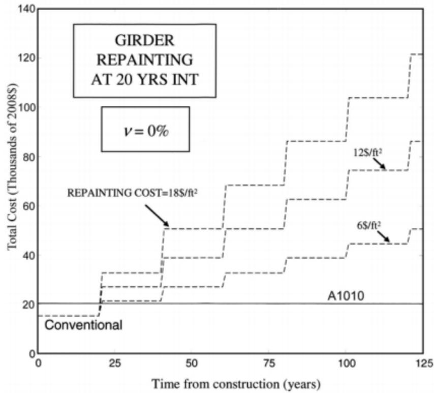
Figure 18 Life cycle cost analysis of difference bridge materials [27]
