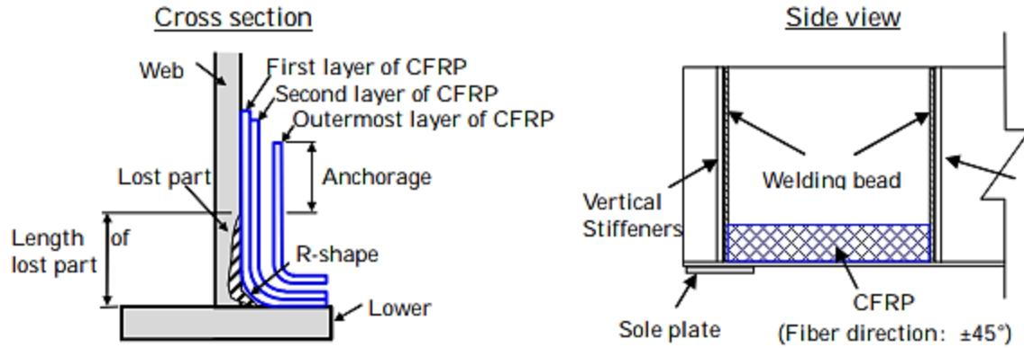
Figure 34 Details of proposed CFRP repair method on corroded webs [57]
