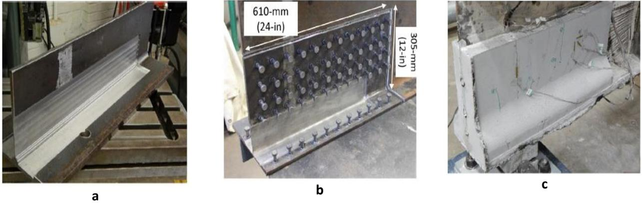
Figure 36 (a) Corrosion simulation on girder; (b) Shear Studs; (c) UHPC Encasement [58]
