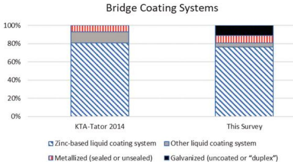
Figure 26 Application popularity of different coating systems [44]
