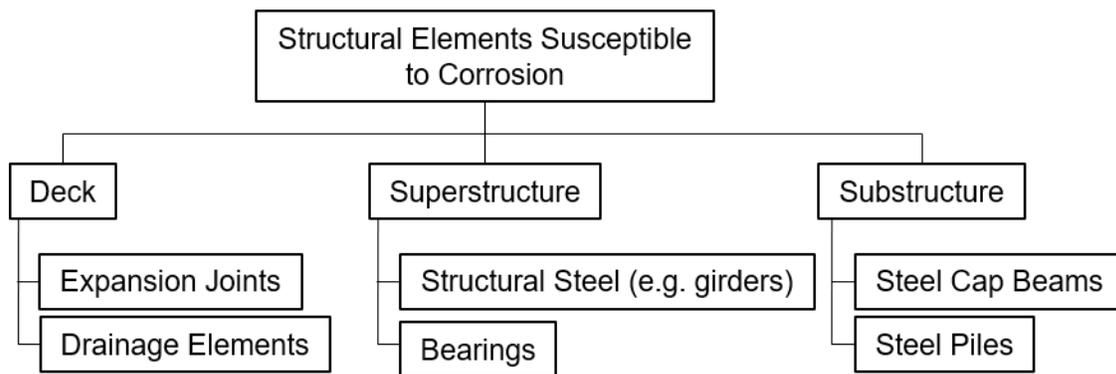
Figure 11. Steel Bridge Components Susceptible to Corrosion (Adapted from [9])
