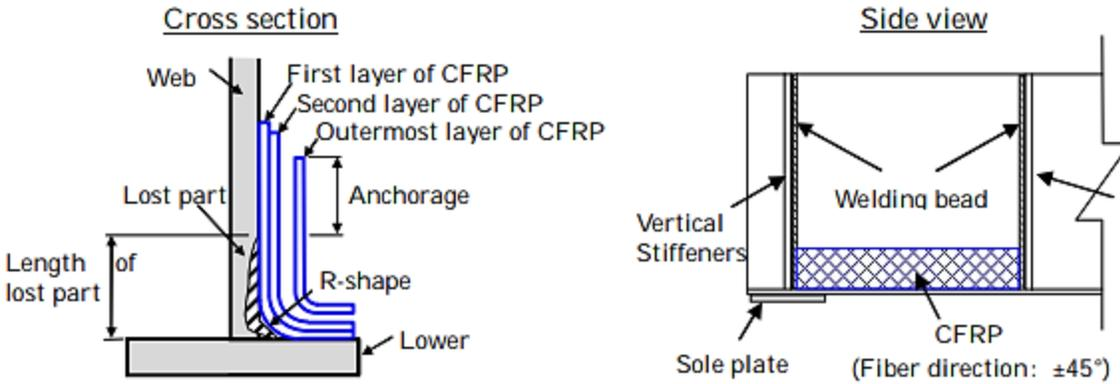
Figure 34 Details of proposed CFRP repair method on corroded webs [57]
