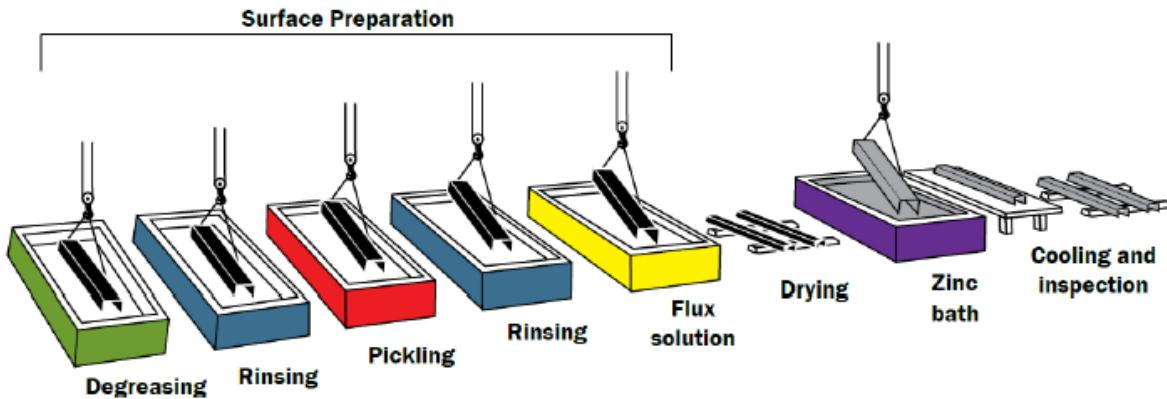
Figure 16. The hot-dip galvanizing process [17]
