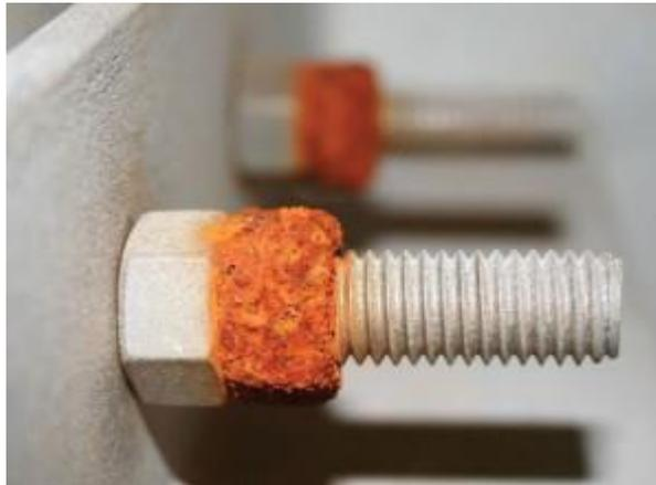
Figure 5. Galvanic Corrosion Resulting from Different Galvanic Potential in the top Nut and Surrounding Metal [8]
