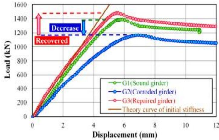
Figure 35 Load-displacement plot for shear buckling tests on corroded girders repaired using CFRP sheets [57]
