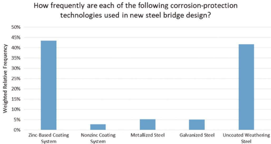
Figure 27 Corrosion protection technologies used for new steel bridges [44]
