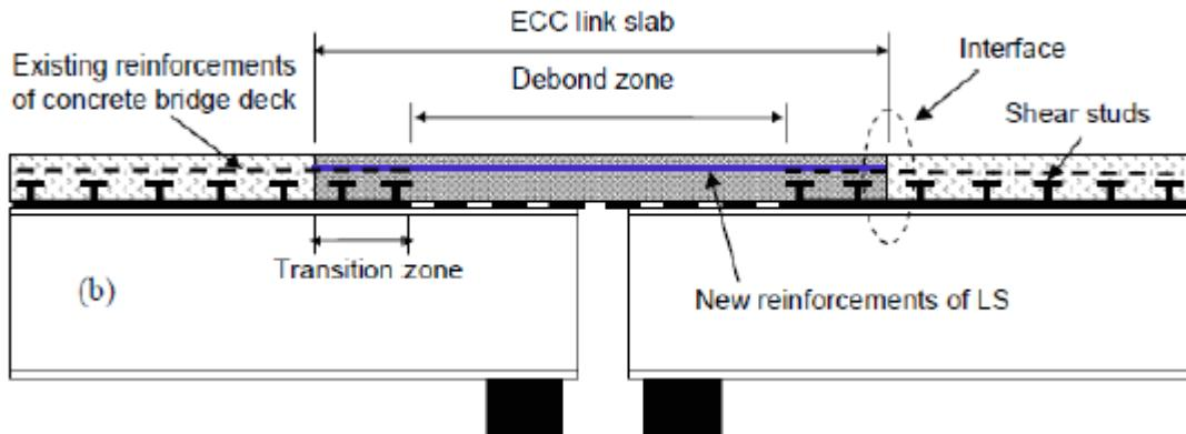
Figure 33 Debonded Link Slab System [54]
