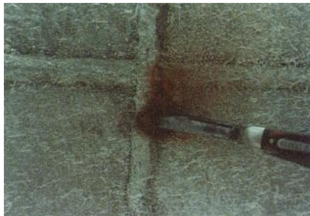
Figure 8. Weld Decay Corrosion [6]
