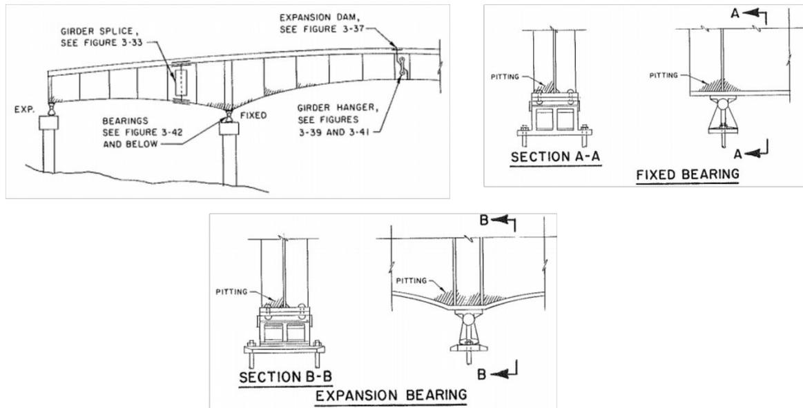
Figure 14. Common Corrosion Patterns in Deck Girder Bridges [6]
