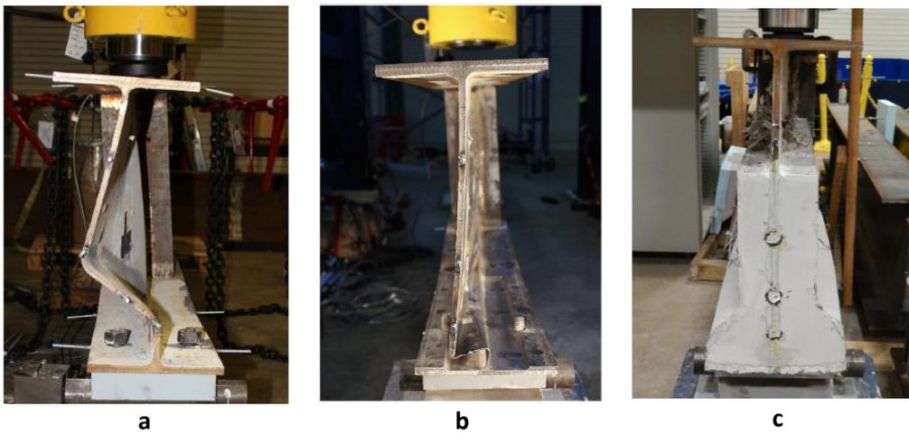
Figure 37 Final conditions of girders showing (a) Web buckling of undamaged girder; (b) localized web buckling of damaged girder; (c) flexural yielding of repaired girder [58]
