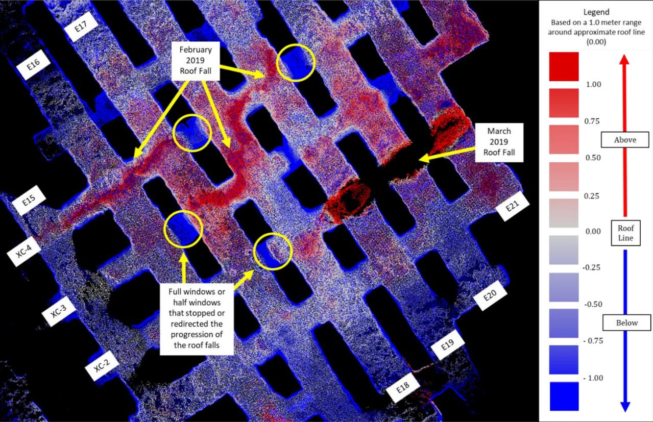
Analysis performed on **one** scan: areas of higher roof elevation (red) indicate damage before scan occurred
