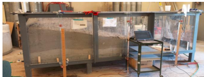
Figure 1: Bench-Scale Assessment of AMD Infiltration in Simulated Highwall Reclaimed with Stabilized FGD Material
