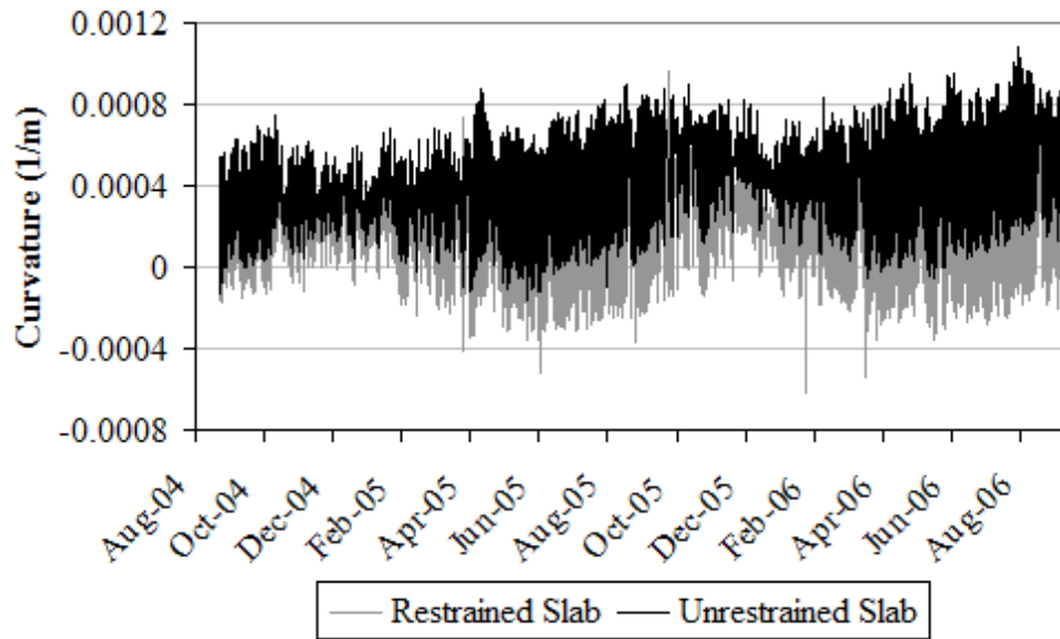
Figure 3. Average slab curvatures for the restrained and unrestrained slabs using computed surface profile measurements from the slab diagonals.
