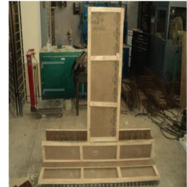
Wood board & contact lumber is selected for casted
