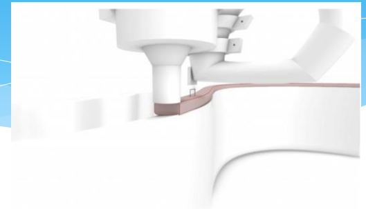
Place steel rope while printing
