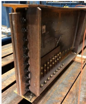
a) bearing region following testing
