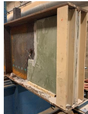
completed FRP repair
