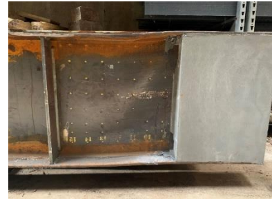
c) observed web buckling behavior (image mirrored)
