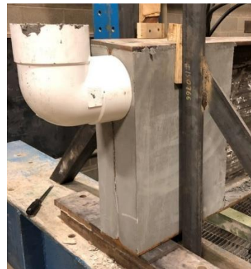
6 in. PVC used to place UHPC
