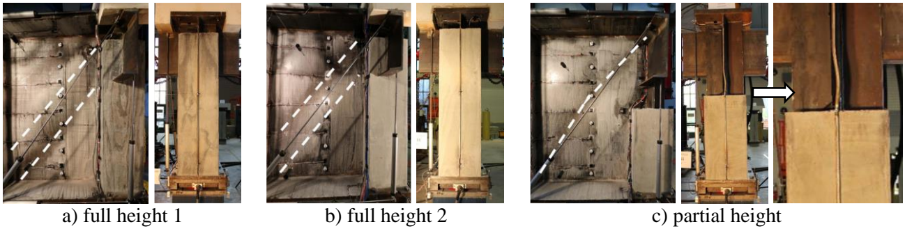
Figure 18 Failure modes of UHPC encased girders reported by McMullen and Zaghi (2020)
