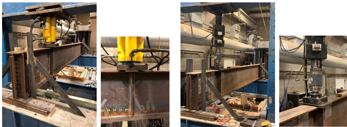
a) Monotonic tests of girder Ends A and B using four 70 kip capacity hydraulic cylinders b) Fatigue conditioning of girder Ends B using 50 kip capacity servo-hydraulic actuator
