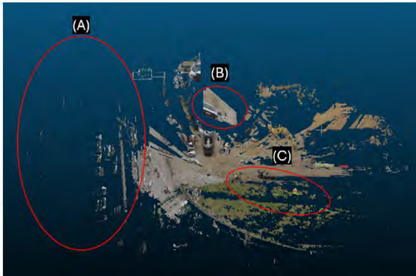
Figure 15: Scan #1/22 with common sources of error highlighted.
