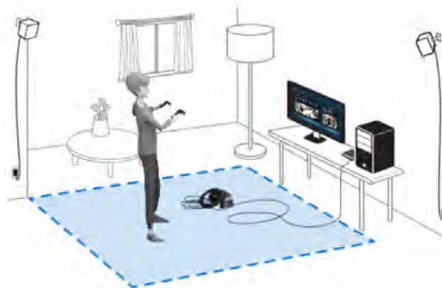
Figure 48: Example of base stations anchoring the corners of the play area. Image from HTC Vive support page [21].
