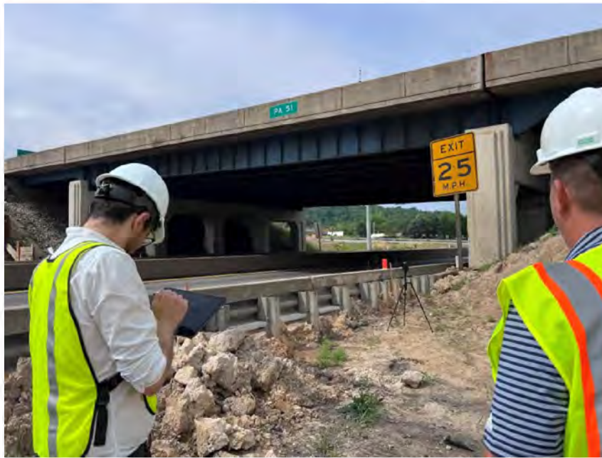
Figure 12: Research team performing a data scanning cycle with the Leica BLK 360.
