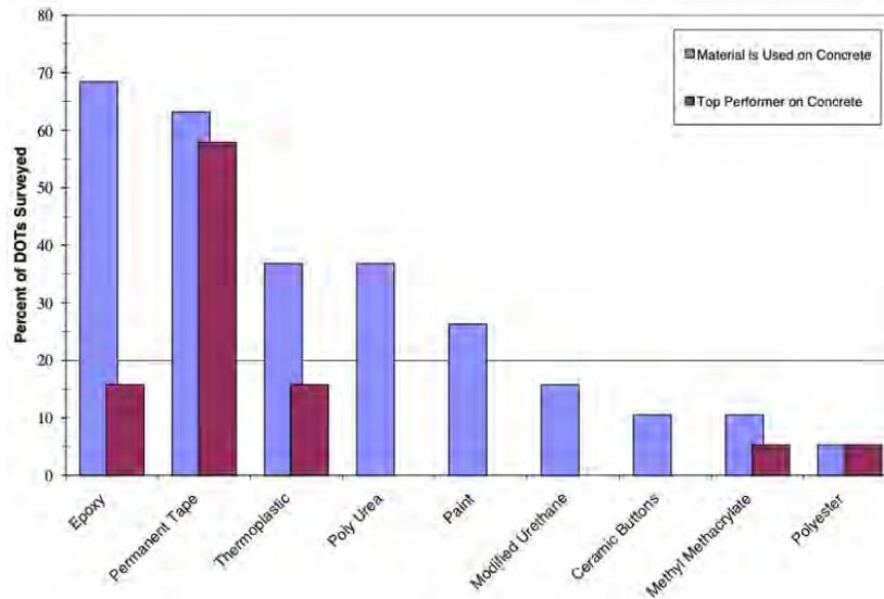
Figure 3: Marking material preference and performance evaluation in PCC pavements by State DOTs [10]
