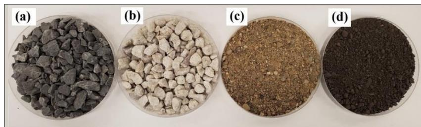
Figure 4. Aggregates. a) #8 Limestone, b) #8 Quartzite, c) Sand, d) Fine LWA
