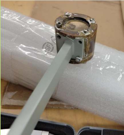
Original K-band rectangular flange
