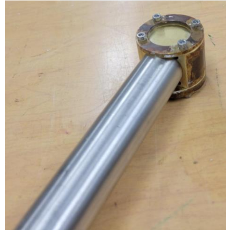
Modified circular-chamfered flange with protective SS316 tube 0.875in diameter and 0.065in wall thickness
