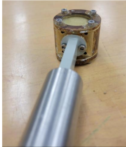
Modified circular-chamfered flange with protective SS316 tube 0.875in diameter and 0.065in wall thickness
