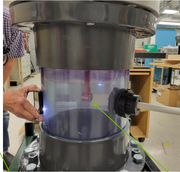
Waveguide insertion probe with cylindrical sensor
