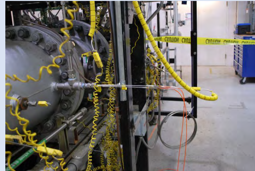
Two fiber-optic probes (sapphire and YAG) & thermocouple (left) and its installation on PPC test rig (right)
