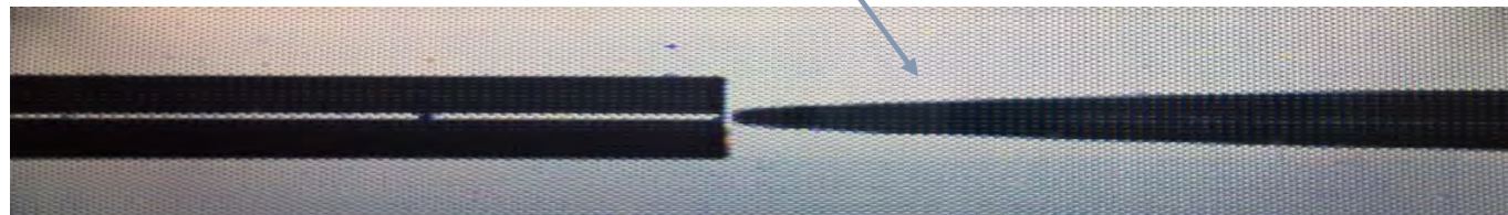
Light coupling between single mode fiber (Left) and sapphire fiber (Right) with the taper tip
