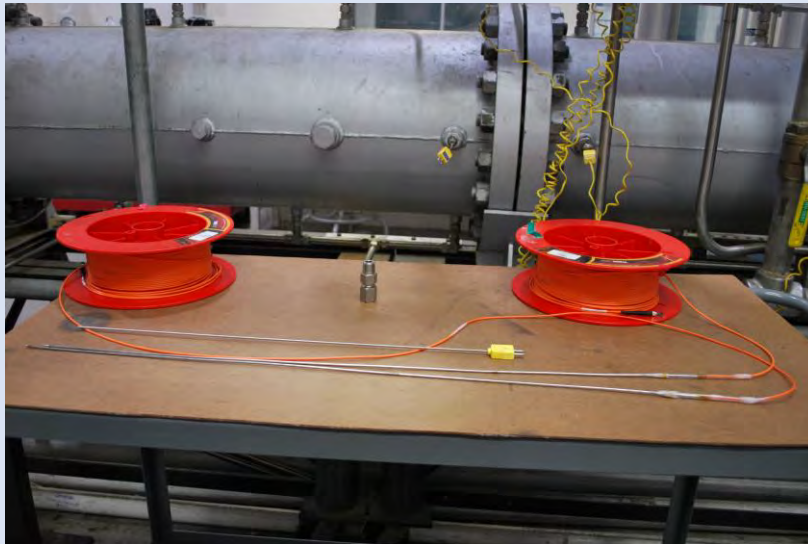
Two fiber-optic probes (sapphire and YAG) & thermocouple (left) and its installation on PPC test rig (right)
