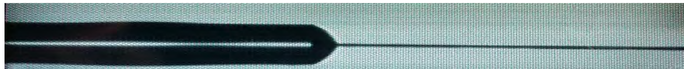
Light coupling between single mode fiber (Left) and silica multimode fiber (Right) with the taper tip
