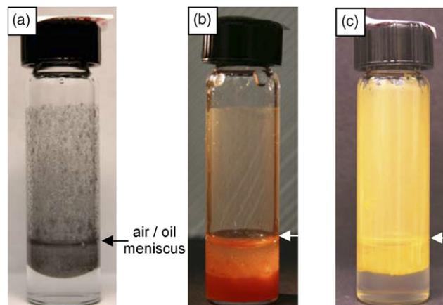
Fig. 4. Climbed films of (a) carbonyl iron particles at oil/water interface, (b)  $\text{Fe}_2\text{O}_3$  particles at oil/water interface, and (c) FeOOH particles at oil/ethylene glycol interface. Arrows show the position of each air/oil meniscus. (For interpretation of the references to colour in this figure legend, the reader is referred to the web version of the article).
