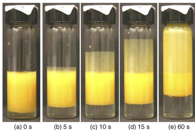
Fig. 2. Sequence of film climbing for FeOOH particles. The time after stopping the shaking of the vial is noted below each image. The change in color intensity from (d) to (e) is attributable to an increase in interfacial concentration of particles in the film with increasing coalescence. (For interpretation of the references to color in this figure legend, the reader is referred to the web version of the article).
