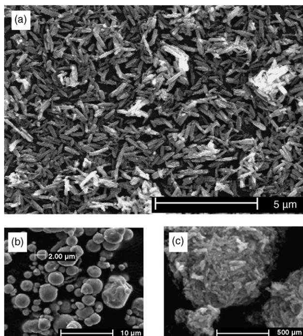
Fig. 1. SEM images of the three types of particles used in the experiment. (a) Iron oxyhydroxide FeOOH, (b) a carbonyl iron (Fe), and (c) iron oxide ( $\text{Fe}_2\text{O}_3$ ).
