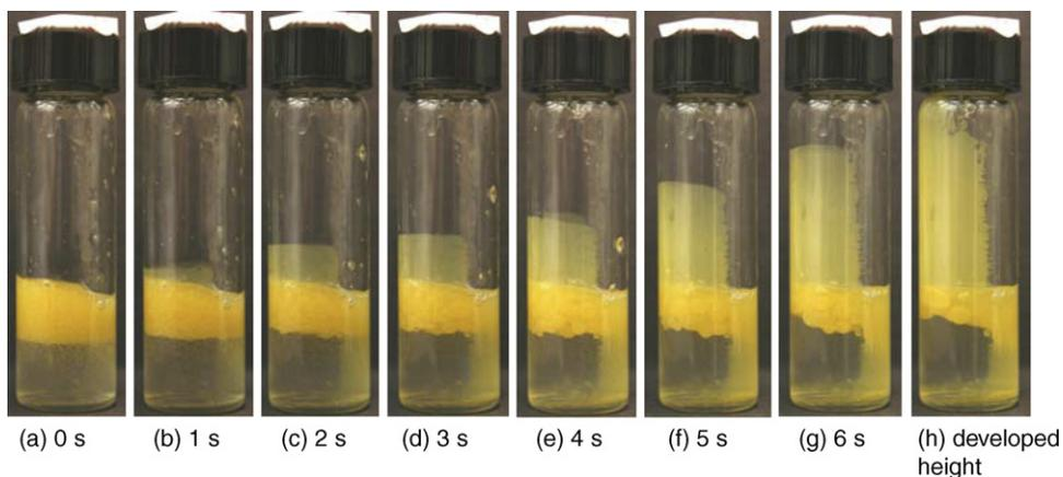
Fig. 8. Effect of hydrophobicity of the walls of the bottle. The time after stopping the shaking of the vial is noted below each image. (For interpretation of the references to color in this figure legend, the reader is referred to the web version of the article).
