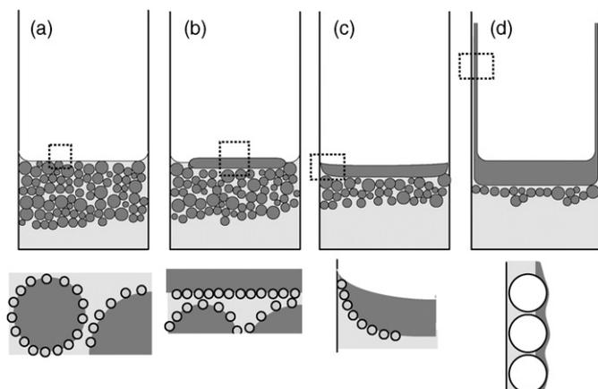
Fig. 3. Schematic of film climbing process. (a) Emulsion after shaking: particles are adsorbed at the interface, (b) drops coalesce and form an oil lens, (c) the lens grows to span the cross-section of the bottle, and (d) particles force the film to climb upwards. In (a)–(d), the region of each dotted rectangle is shown in magnified form below each figure.
