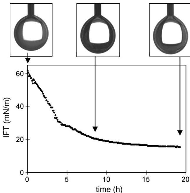
Fig. 7. Interfacial tension (IFT) vs. time, and corresponding pendant drop shapes at  $t=0$ ,  $t=8.33$  h, and  $t=18.6$  h.
